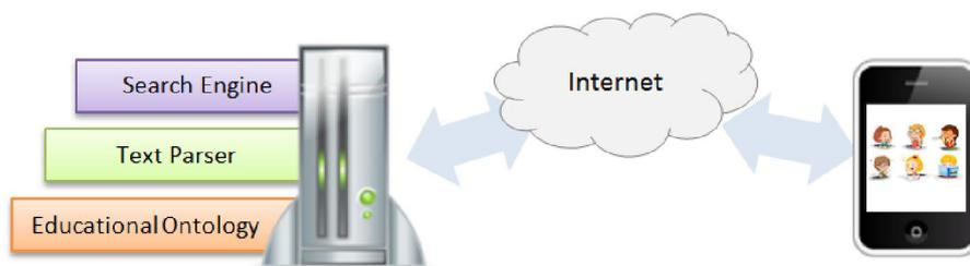
Fig. 8: System architecture
