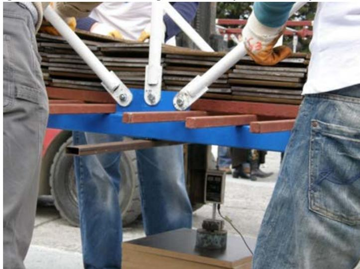
Figure 4. Application of the Vertical Loads to the Bridge.
